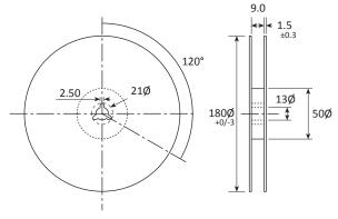
Not to scale. Dimensions in mm. Tolerances ±0.1mm unless otherwise stated.
