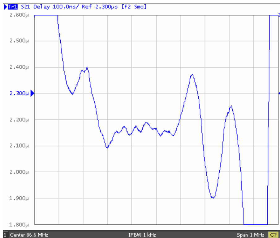
Fig-3 Group Delay Ripple: Horizontal: 0.1MHz/Div Vertical:100nS/Div
